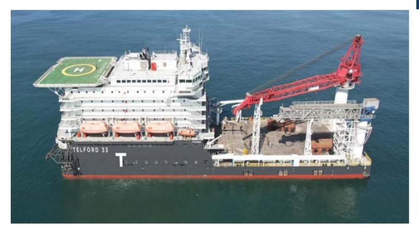
The vessel, a 2021-built DP3 Multi-Purpose Support Vessel (MPSV), provides accommodation for up to 684 persons and available free deck space of 2,000m2. It is equipped with a 300-tonne heavy-duty crane and a heave-compensated gangway, making it a highly versatile addition to the fleet
