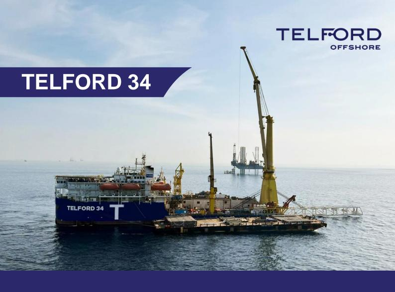
Built according to a distinctive hybrid design philosophy, the multipurpose Telford 34 DP3 vessel includes a large unobstructed deck, an 800mT capacity crane with active heave compensated (AHC) features, a heave compensated gangway and a modular rigid/flexible pipelay system.
