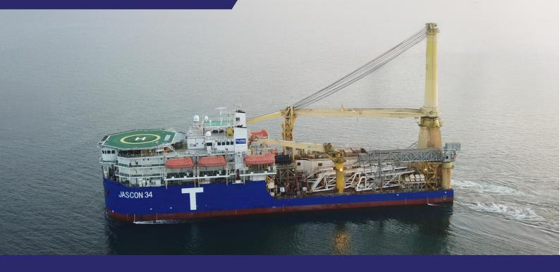
Built according to a distinctive hybrid design philosophy, the multipurpose Telford 34 DP3 vessel includes a large unobstructed deck, an 800mT capacity crane with active heave compensated (AHC) features, a heave compensated gangway and a modular rigid/flexible pipelay system.
