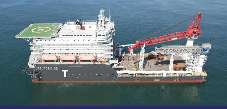
Built according to a distinctive hybrid design philosophy, the Telford 33 is a multipurpose DP3 vessel suitable for offshore accommodation, hook up and construction activities. The Telford 33 has accommodation for 684 persons, a large 2000m<sup>2</sup> deck, and a 300mt crane. The vessel is also equipped with a Kongsberg DP3 K-POS 22/12 system including follow target mode and an active heave-compensated hydraulic telescopic gangway.
