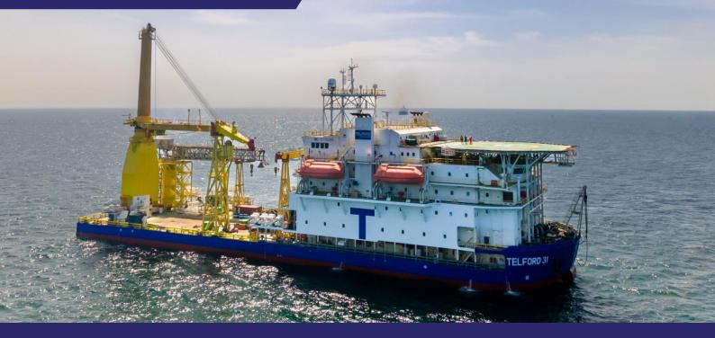
Built according to a distinctive hybrid design philosophy, the Telford 31 combines strong offshore construction capability with high accommodation capacity. With 1300m<sup>2</sup> of unobstructed deck area and a 400mt capacity active heave-compensated (AHC) subsea crane, she offers extensive subsea support services for a wide variety of projects.
