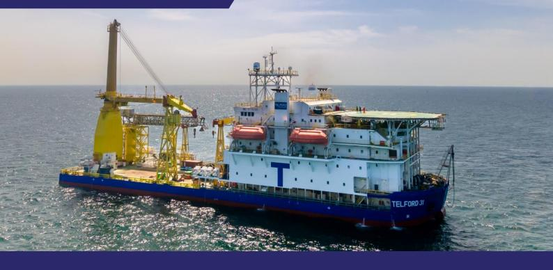
Built according to a distinctive hybrid design philosophy, the Telford 31 combines strong offshore construction capability with high accommodation capacity. With 1300m<sup>2</sup> of unobstructed deck area and a 400mt capacity active heave-compensated (AHC) subsea crane, she offers extensive subsea support services for a wide variety of projects.
