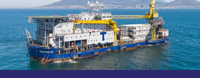
Built according to a distinctive hybrid design philosophy, the Telford 30 is a multipurpose DP3 vessel suitable for offshore accommodation, hook up and construction activities. The Telford 30 vessel has a large unobstructed main deck, a 270mt crane and large-scale accommodation capacity.
