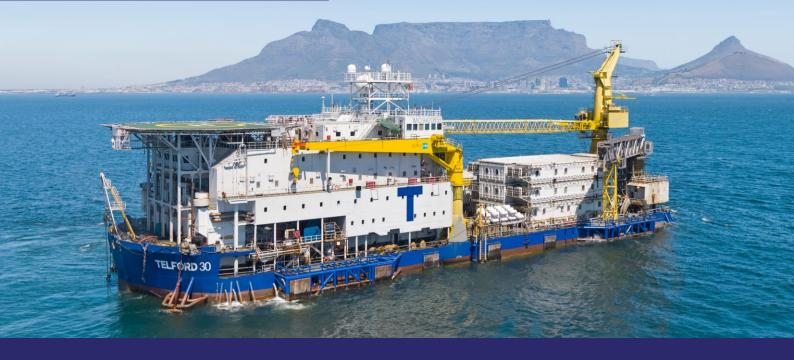
Built according to a distinctive hybrid design philosophy, the Telford 30 is a multipurpose DP3 vessel suitable for offshore accommodation, hook up and construction activities. The Telford 30 vessel has a large unobstructed main deck, a 270mt crane and large-scale accommodation capacity.
