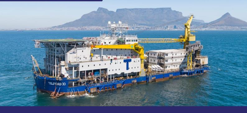
Built according to a distinctive hybrid design philosophy, the Telford 30 is a multipurpose DP3 vessel suitable for rigid pipelay, offshore construction and accommodation and hook up activities. The Telford 30 vessel has a large unobstructed main deck, a 270mt crane and large-scale accommodation capacity.
