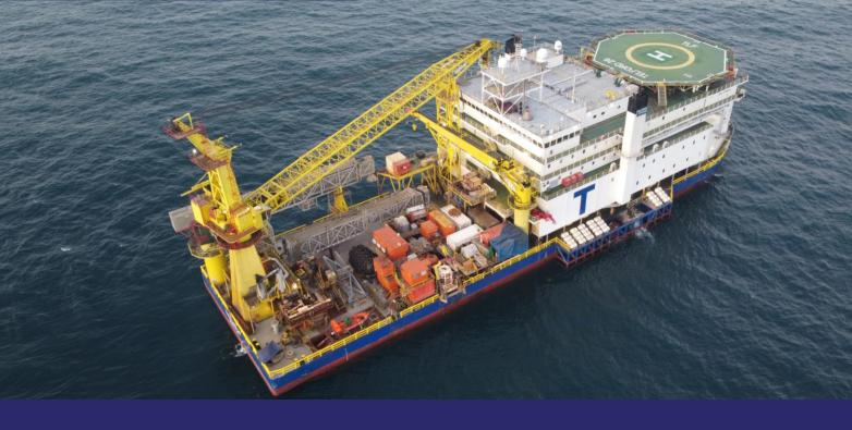
Built according to a distinctive hybrid design philosophy, the multipurpose Telford 28 DP3 vessel is equipped with a heave-compensated gangway, a large deck space and a 270mt crane. The Telford 28 is an ideal vessel for accommodation and hook up activities where high-capacity POB and a large and versatile deck space are required.
