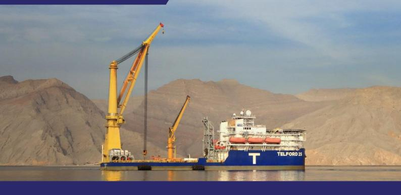
Built according to a distinctive hybrid design philosophy, the multipurpose Telford 25 DP3 vessel includes a large unobstructed deck, an 800mt capacity crane with active heave compensated (AHC) features, a heave compensated gangway and the option of installing a modular rigid/flexible pipelay system.
